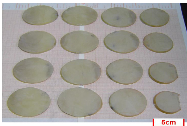
Fig. 6. [001]-oriented crystal plates cut from PIMNT crystal boule.
